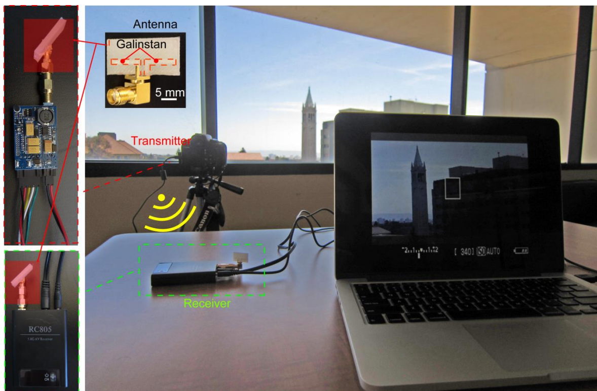
Figure S4. Wireless transmission of video content from a camera to a laptop using 24.5 mm dipole antennas installed into a video receiver and transmitter. Left side images in boxes are top views of the transmitter and receiver with liquid dipole antennas.
