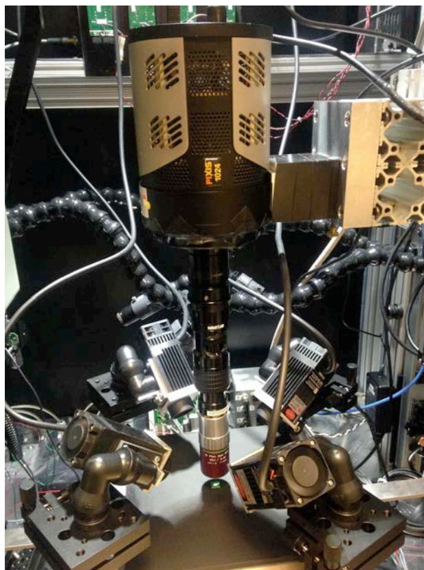
Fig. 2. Photograph of the PL imaging experimental setup showing the PIXIS camera with Navitar and Mitutoyo lens system for close up zoom and high spatial resolution.
