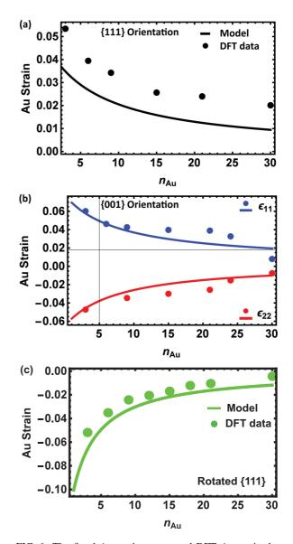
FIG. 6. The fitted Au strain curves and DFT Au strain data as a function of Au layer number for (a) the biaxial tensile strain in  $\{111\}$  orientation, (b) he two in-plane strains in  $\{001\}$  orientation, and (c) the biaxial compression strain in rotated  $\{111\}$  orientation.
