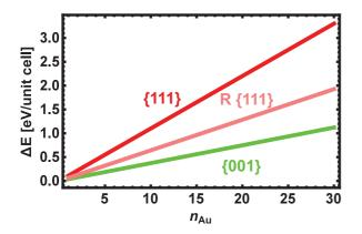
FIG. 2. The strain energy per unit cell for Au deposition on  $MoS_2$ in three orientations computed assuming that the  $MoS_2$  is unrelaxed, and that surface and interfacial energies make negligible contributions to the energy. The rotated {111} orientation is labeled as "R {111}."
