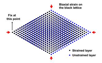
FIG. 3. The two layer  $MoS_2$  system (top view). Only the lattice points are shown. The black points indicate the first layer that has 5% biaxial strain. The blue points indicate the second layer, which is without the strain. The lattice points of the two layers also coincide at the corners of the strained layer.
