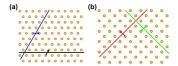
FIG. 4. (a) The dislocation geometry in Au {111} and rotated {111} orientations. The straight lines indicate the line direction. The arrows with same color give the corresponding Burger's vectors (in rotated {111} the Burger's vectors are in opposite direction). The two sets of the dislocations have same spacing. (b) The dislocation geometry in Au {001} orientation film. There is no direct constraint between the spacing of the two sets.
