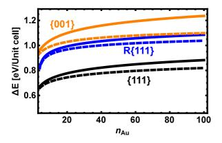
FIG. 7. The  $\Delta E$  of the epitaxy systems with and without compliant substrate (but all with surface/interface energies and misfit dislocations). The dashed lines are the curves for the systems with compliant substrate and the solid lines are for those without compliant substrate. Enabling compliant substrate does lower the energy. In addition, this reduction increases as the Au film grows.
