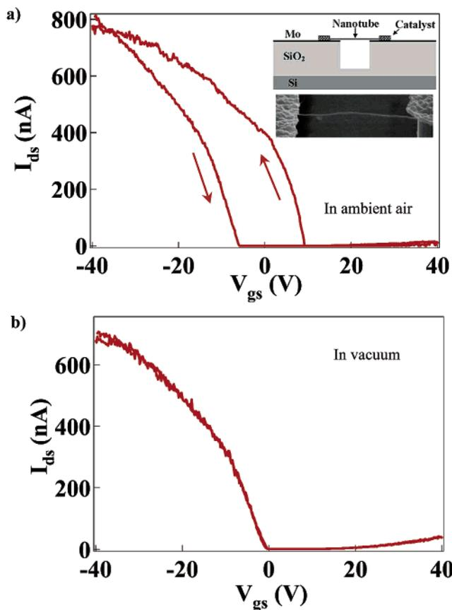
**Figure 3.** (a)  $I_{ds}$ - $V_{gs}$  curves recorded for a suspended SWNT FET exposed to ambient air. Bias voltage  $V_{ds} = 10$  mV.  $V_{gs}$  sweep rate = 0.1 V/s. The inset shows a scanning electron microscopy image and a schematic structure of the device. (b) Diminished hysteresis recorded with the same device immediately after placing it in vacuum.
