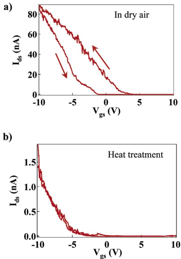
**Figure 4.** (a)  $I_{ds}$ - $V_{gs}$  data for an SWNT FET (on  $\text{SiO}_2$ ) in dry air.  $V_{ds} = 10$  mV. (b) Significantly reduced hysteresis recorded for the device after heating to  $200^\circ\text{C}$  in  $\text{H}_2$  for 4.5 h, cooled to room temperature, and exposed to dry air for 5 h. The schematic drawing depicts the removal of surface-bound water after the thermal treatment.
