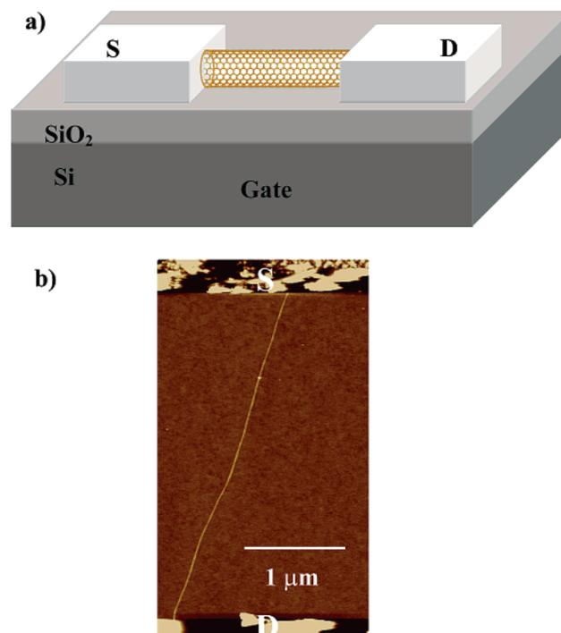
**Figure 1.** (a) Schematic structure of a back-gated SWNT FET. (b) Atomic force microscopy image of a device with a single nanotube (lying on SiO<sub>2</sub>) bridging source (S) and drain (D) electrodes.
