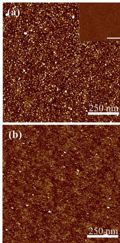
**Figure 1.** AFM images of (a) nanoparticles formed on SiO<sub>2</sub> after soaking in the hydroxylamine/FeCl<sub>3</sub> solution for 2 min and (b) iron-oxide nanoparticles after calcination in air at 800 °C for 5 min, respectively. The inset in (a) shows a bare SiO<sub>2</sub> surface and the scale bar is 1 μm.
