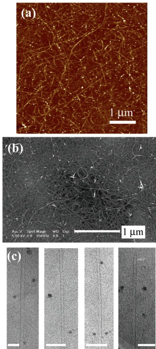
**Figure 2.** (a) AFM and (b) SEM images of SWNT films grown from a near-monolayer of catalyst nanoparticles on SiO<sub>2</sub> via hydroxylamine assisted deposition. (c) Several TEM images of individual SWNTs grown on SiO<sub>2</sub> TEM grids. The back-ground is the 10 nm thick SiO<sub>2</sub> film and appears somewhat granular. Scale bars: 5 nm.
