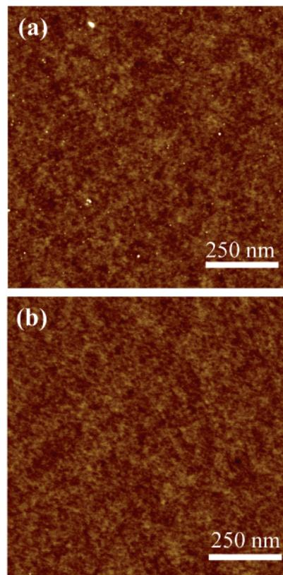
**Figure 5.** AFM images of hydroxylated SiO<sub>2</sub> surfaces after soaking in hydroxylamine/FeCl<sub>3</sub> solution for 2 min, the solution pH is (a) 2.3 and (b) 10, respectively.
