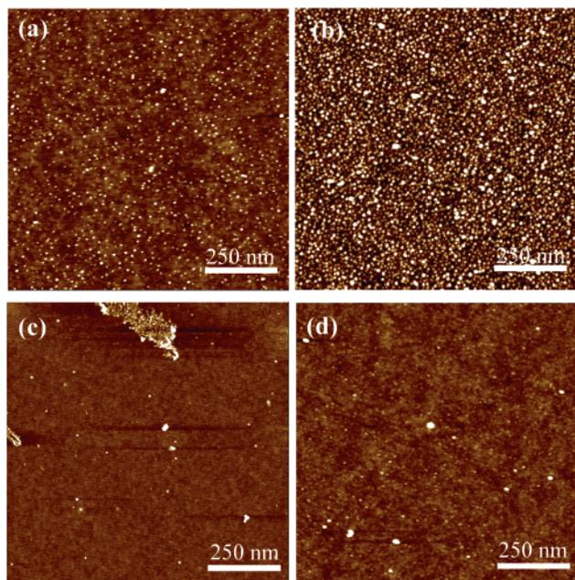
**Figure 4.** AFM images of hydroxylated SiO<sub>2</sub> surfaces after soaking for (a) 10 s and (b) 5 min respectively in the hydroxylamine/FeCl<sub>3</sub> solution. (c) An AFM image showing no systematic particle formation on a SiO<sub>2</sub> substrate without hydroxylamine in the solution. (d) An AFM image showing less particle deposition on a SiO<sub>2</sub> substrate after removal of surface hydroxyl group by high-temperature annealing.
