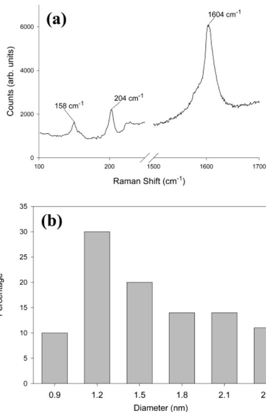
**Figure 3.** (a) Representative micro-Raman spectroscopy of SWNTs in a 1 μm<sup>2</sup> area of SiO<sub>2</sub>. (b) Nanotube diameter distribution measured from resonance micro-Raman data.
