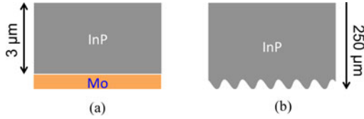
Fig. 6. Overall structure for the two samples investigated in this study. (a) VLS-grown InP thin film on top of a Molybdenum substrate and (b) InP wafer that is 250 \mu\text{m} thick.
