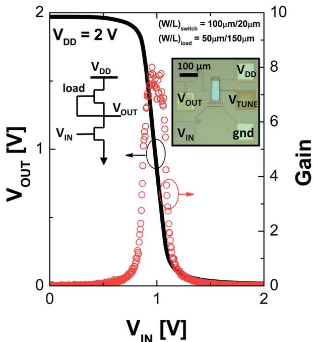
**Figure 5.** Voltage transfer curve ( $V_{OUT}$  vs  $V_{IN}$ ) and DC gain ( $\partial V_{OUT}/\partial V_{IN}$ ) of the all-oxide NMOS inverter on polyimide under an operation voltage  $V_{DD} = 2$  V. The switching transistor has a  $W/L = 100 \mu\text{m}/20 \mu\text{m}$ , and the depletion-mode load transistor has a  $W/L = 50 \mu\text{m}/150 \mu\text{m}$ . Inset is a schematic representing the device layout as well as the corresponding optical image of the device with labeled contacts.
