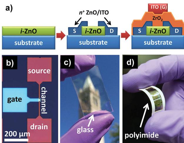
**Figure 1.** a) Process schematics of ZnO TFT fabrication. b) Optical microscope image of finished device on silicon. c) Photograph of finished device array on glass slide. d) Photograph of finished devices on freestanding polyimide foil bent between fingers.
