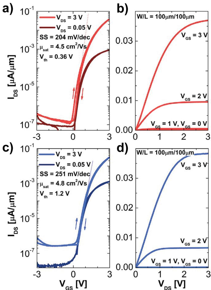
**Figure 3.**  $I_{DS}$ - $V_{GS}$  and  $I_{DS}$ - $V_{DS}$  curves for  $W/L = 100 \mu\text{m}/100 \mu\text{m}$  device on a,b) alkali-free glass and c,d) polyimide. The arrows on the transfer curves indicate the direction of the double sweep measurement.
