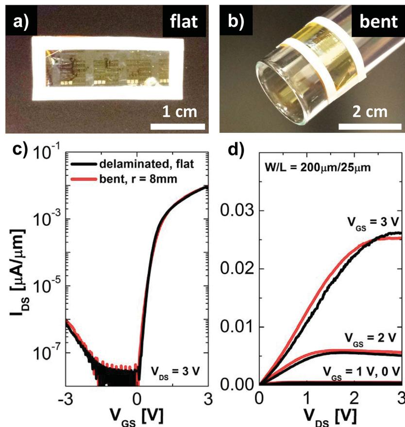
**Figure 4.** Photographs of the substrate while a) flat and b) bent around a test tube with  $r = 8$  mm. c)  $I_{DS}-V_{GS}$  and d)  $I_{DS}-V_{DS}$  curves for  $W/L = 200 \mu\text{m}/25 \mu\text{m}$  device on freestanding polyimide (black) and bent at  $r = 8$  mm (red).
