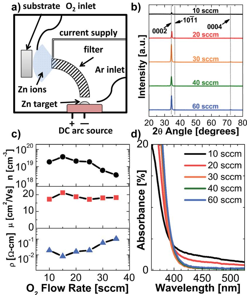
**Figure 2.** a) Schematic of cathodic arc deposition chamber. The permanent magnet is denoted in red. b) XRD spectra for ZnO films deposited at different O<sub>2</sub> flow rates. c) Electron concentration ( $n$ ), Hall mobility ( $\mu$ ), and resistivity ( $\rho$ ) as a function of O<sub>2</sub> flow rate. d) Dependence of optical absorption with O<sub>2</sub> flow rate.
