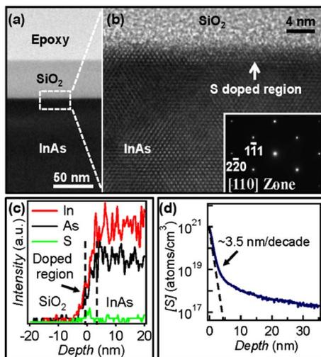
FIG. 3. (Color online) Structural and chemical profiling of S-doped InAs using an annealing condition of 450 °C for 300 s. [(a) and (b)] Low and high resolution TEM images showing SiO<sub>2</sub>/S-doped InAs interfaces. The ~4 nm dark contrast region corresponds to the S-doped layer. (c) EDS demonstrating the In, As, and S chemical profiles across the junction interface. (d) SIMS profile of S in InAs. The profile abruptness is ~3.5 nm/decade near the doped surface region.
