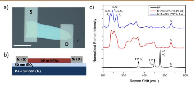
Figure 1. (a) Optical microscope image of a typical b-P gated photoconductor with a thickness of 29 nm; the scale bar is  $10 \,\mu\text{m}$ . (b) Cross-sectional schematic of the gated photoconductor. (c) Raman spectra measured for pure b-P as well as b-PAs alloys.
