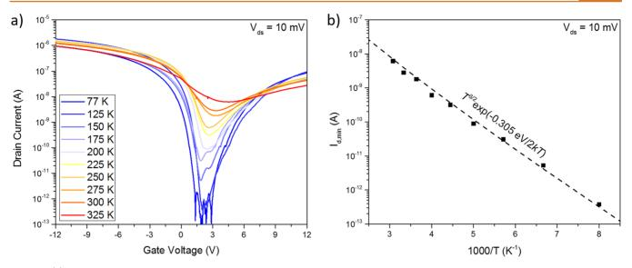
Figure 3. (a) Transfer characteristics of an 18 nm-thick b-P crystal measured as a function of temperature at a drain bias of 10 mV. Note that a cold shield was utilized for these measurements. (b) Arrhenius plot of minimum drain source current  $(I_{d,min})$  as a function of temperature extracted from panel (a). Dashed line is a fit based on G-R limited dark current.
