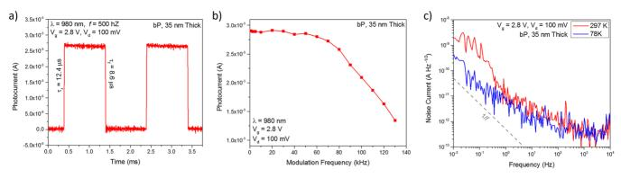
Figure 5. (a) Room-temperature temporal photoresponse of a 35 nm-thick b-P photoconductor, excited by a 980 nm laser modulated at 50 kHz. (b) Photocurrent *versus* modulation frequency measured at an incident power of 15 nW measured at room temperature, showing a 3 dB frequency of 117 kHz. (c) Noise spectrum measured for a 35 nm-thick b-P photoconductor at room temperature and 77 K; dashed line shows a reference 1/f curve.
