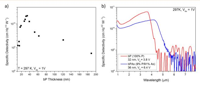
Figure 7. (a) Specific detectivity of b-P photoconductors as a function of layer thickness; measurements were performed under gating conditions which maximized the detectivity for the specific device at room temperature. (b) Specific detectivity of b-P and b-PAs photoconductors with optimized thickness; measurements were performed under gating conditions which maximized detectivity for the specific device at room temperature.
