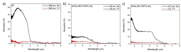
**Figure S2.** (a) Absorption spectra, calculated from 100-T-R in the X and Y directions measured on 348 nm thick b-P. (b) Absorption spectra, calculated from 100-T-R in the X and Y directions measured on 26 nm thick b-PAs (83% As). (c) Absorption spectra, calculated from 100-T-R in the X and Y directions measured on 212 nm thick b-PAs (91% As). Note that the total absorption is a strong function b-P/b-PAs thickness and refractive index.
