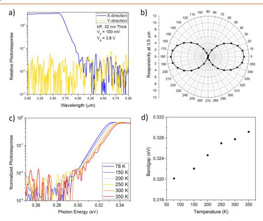
Figure 6. (a) Relative response of a b-P photoconductor measured for incident light polarized along (x-direction, arm-chair) and perpendicular to (y-direction, zigzag) the absorbing axis of the b-P crystal. (b) Responsivity of the device shown in panel (a) as a function of polarizer angle. (c) Normalized photoresponse of a b-P photodetector measured as a function of temperature. (d) Extracted bandgap from the spectral photoresponse as a function of device temperature.
